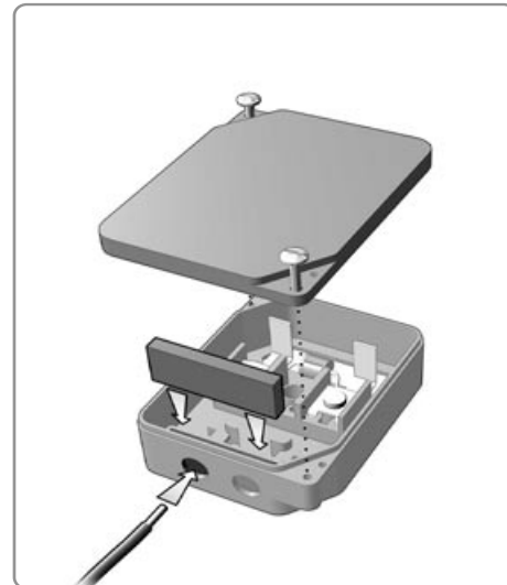
Wiring ProCharger™-S-junction box
